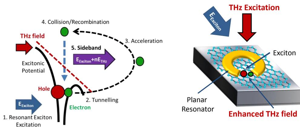
**Schematic of High Sideband Generation.** A resonant excitation of the exciton is driven by a THz excitation. The electron is separated from the hole by the THz field followed by a collision with a hole that releases a high energy sideband.
